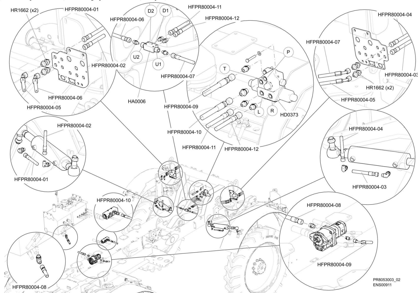
Direction standard 2RD – Standard Steering for 2WS
