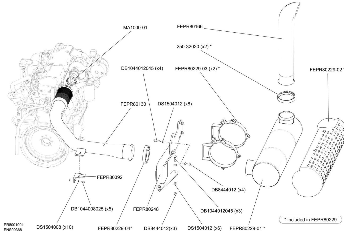
Circuit gasoil T4F - Diesel circuit T4F
