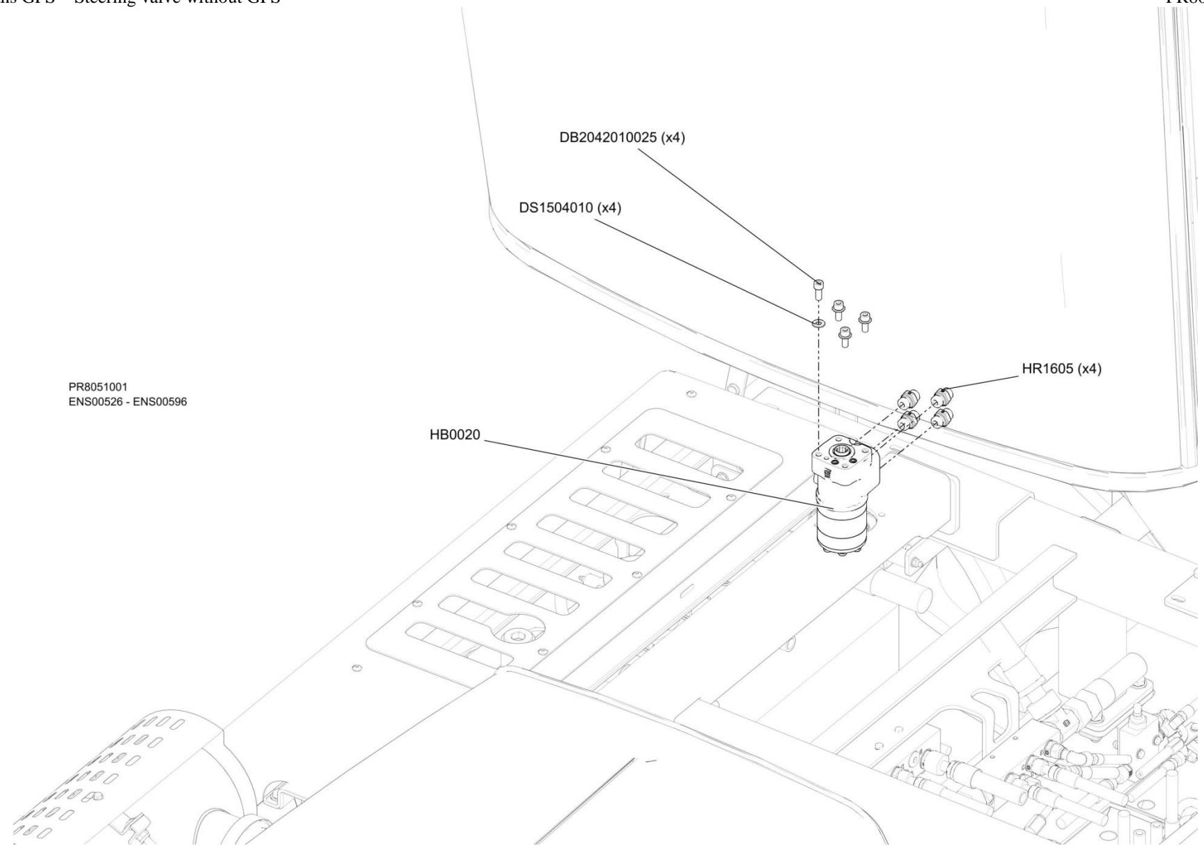
Circuit hydraulique Direction 2RD – Hydraulic Steering Circuit for 2 WS
