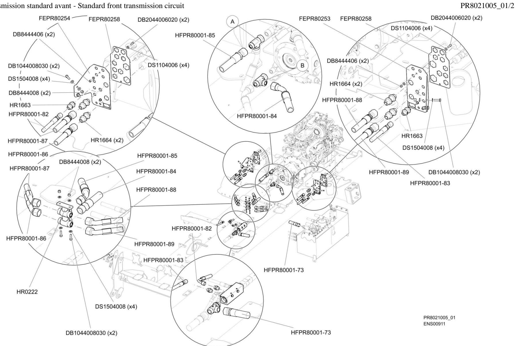
Circuit transmission standard avant - Standard front transmission circuit
