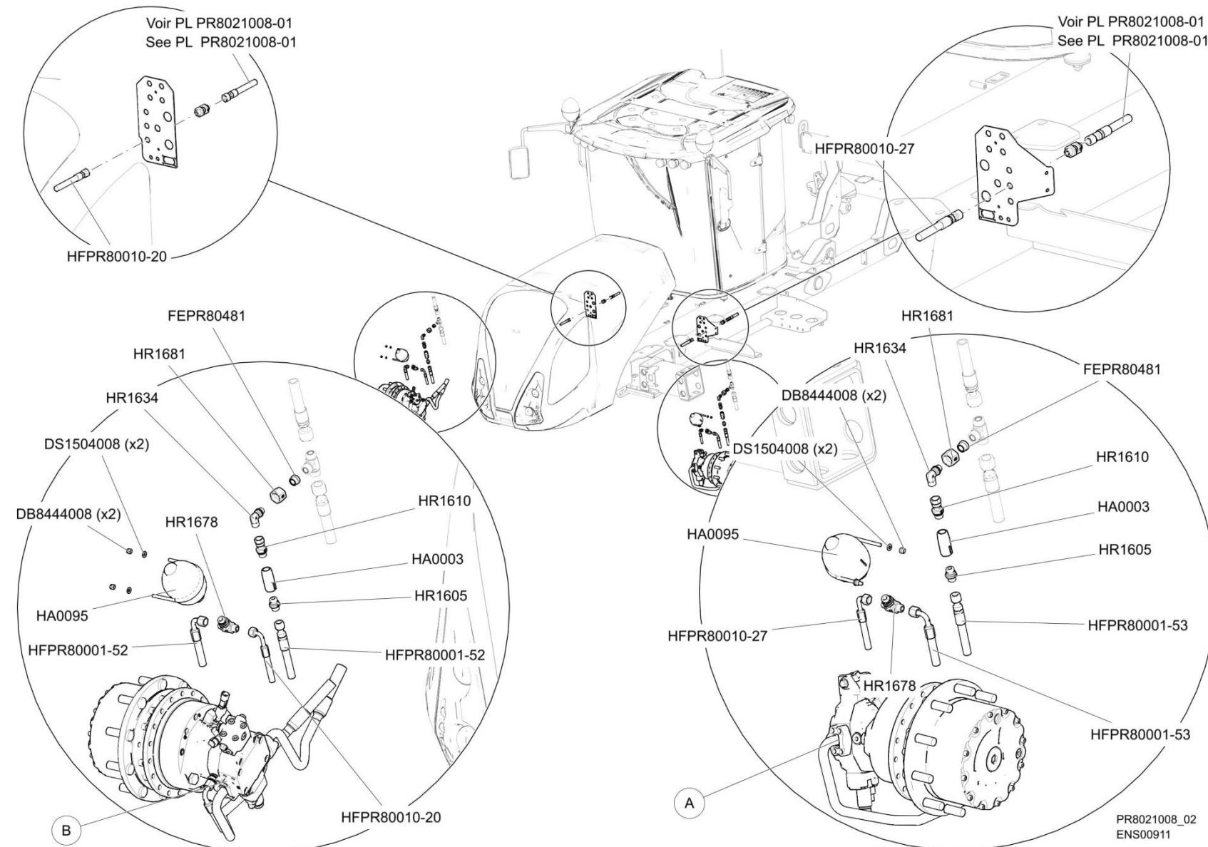
Circuit gavage sur essieu arrière – Boost Pump circuit of the Rear Axle
